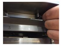
3. Remove the crossfire panel. The crossfire panel is a downward U shaped channel located between the burners towards the rear of the burners. The crossfire panel is removed by unscrewing the fastener under the channel which holds it in place. The most commonly used fastener can be removed with a metric #4 Allen wrench included with the sear burner.
