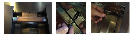
4. Install the infrared burner into the grill in the same way that the conventional burner installed with the male post on the rear of the burner resting in the opening in the grill chassis and the cylindrical venture tube installing around the valve stem in the front. Note: IT IS CRITICAL THAT THE FRONT END OF THE INFRARED BURNER IS INSTALLED APPROPRIATELY ONTO THE GAS VALVE TO ENSURE THE GAS FLOWS SAFELY INTO THE BURNER.
